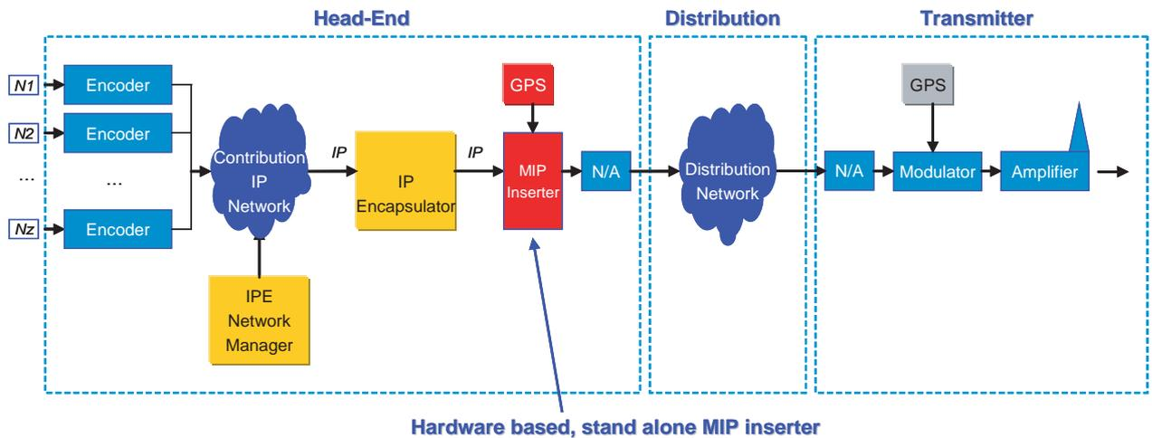
**Figure 1 - Traditional architecture with MIP in separate device**
